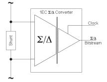
THE CLT IS WELL PROVEN in IGBT-Drivers and forms with the Sigma-Delta technology an interface to the integrated shunt. The task to be completed by this interface is to read out the electric value, transform it to digital information and transmit this information to the controller level providing galvanic isolation.
